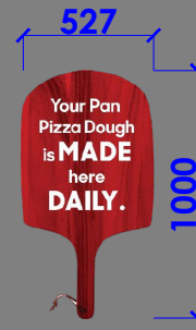
PLOTTER CUT VINYL/CLEAR PRINTED LETTER TO BE PASTED ON 10MM THK ROUTER CUT MDF
