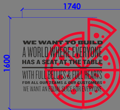
RED HAND PAINTED PIZZA ARTWORK & 10 MM THK ROUTER CUT BLACK ACRYLIC LETTERS
