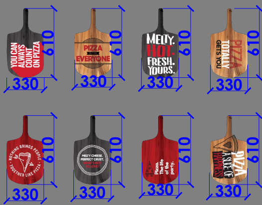
PLOTTER CUT VINYL/CLEAR PRINTED LETTER TO BE PASTED ON 10MM THK ROUTER CUT MDF PAN
