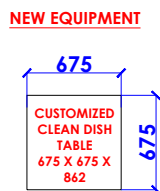
(13) CLEAN DISH TABLE WITH 2 U/S : 01 NOS. HEIGHT 862mm HT
