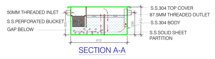
PORTABLE GREASE TRAP DETAILS
