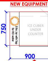
(4) BEVERAGE TABLE WITHOUT SINK + WITH 1 TROLLEY WITH WHEELS OF 3" HEIGHT FOR ICM : 01 NOS. HEIGHT 1016mm HT
