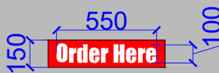
ORDER HERE LETTERS IN WHITE ACRYLIC-PASTED ON RED PORTAL FINISHED WITH LUSTER PAINT - SIGNAL RED 0520 DUCO PAINT -1 NOS.
