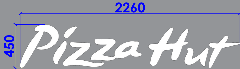
ENGLISH LETTERS- PIZZA HUT- 3D BACKLIT LETTERS 450MM HT FOR FRONT FACADE
